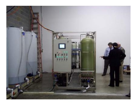
**WaterSafe CS60**, a larger stationary configuration (shown below) provides 15,000 gallons / 57,000 liters/ 57 m3 per day. This unit pictured below is currently located in the earthquake zone in Sichuan, China.
